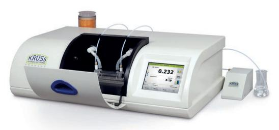
Semi-automatic sample supply with P8000-TF and peristaltic pump DS7070
