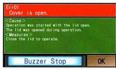
Error details, explanation of cause, and recommended action are displayed together with the error number.
