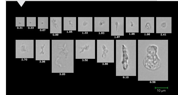
PARTICULATE WITHIN A PARENTERAL DRUG, RANGING FROM 310 nm TO 9.6 µm IN SIZE, AS **IMAGED BY THE FLOWCAM** NANO. DIAMETER (µm) OF EACH PARTICLE IS NOTED BENEATH EACH IMAGE. PARTICLES CAN BE SORTED BY 40+ PARAMETERS, INCLUDING **MORPHOLOGICAL** CHARACTERISTICS, USING VISUALSPREADSHEET.
