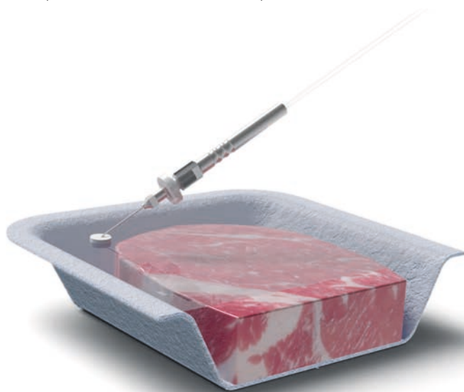
Taking a protective gas mixture sample from a food package
