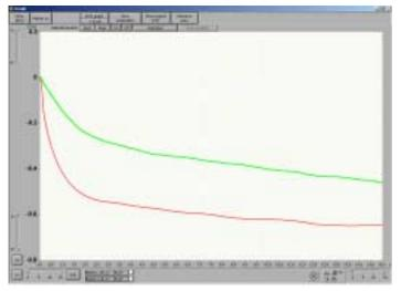
Shrinkage of two different LWC papers with 50% relative moistness at a temperature of  $130^{\circ}C$
