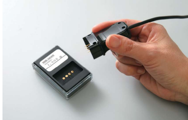
●Check probes by Probe checker prior to measurements
