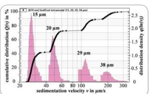
Particle velocity distribution of a suspension made from batches of 4 monodisperse PMMA reference particles (nominal size indicated, LUMiReader PSA, 120 profiles,  $\Delta t = 20 \text{ s}$ ,  $T = 30^{\circ}\text{C}$ ,  $\lambda = 870 \text{ nm}$ ).
