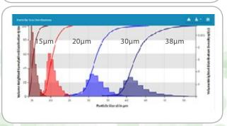
Transmission profile and corresponding particle size distribution of 4-modal PMMA reference particles
