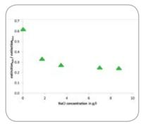
Agglomeration detected, extinction of Ludox 45 nm for different wavelengths in dependency time & ionic strength
