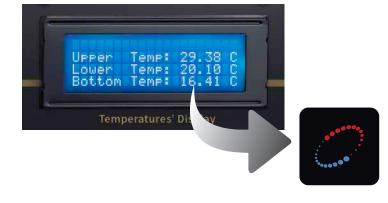
Once stable, temperatures from upper temperature ( $T_{\rm u}$ ), lower temperature ( $T_{\rm L}$ ) and heat sink temperature ( $T_{\rm H}$ ) are then entered into the GHFM-02 software for auto calculation of thermal resistance, and calibrated thermal conductivity results.
