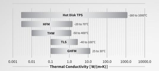
Thermtest has been advancing the measurement of thermal conductivity, thermal diffusivity, and specific heat for more than a decade. With more than 2000 satisfied customers worldwide, our unique combination of advanced thermal conductivity instrumentation for the laboratory, portable meters for the field, and accessories, enables us to provide ideal solutions to fit any material testing application and budget.
