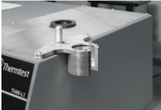
Vertical cell mount attached without sample.
