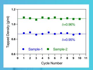
The 10 cycle measurements of two samples demonstrate the excellent **repeatability** (<1.0%) of the BeDensi T Pro Series.
