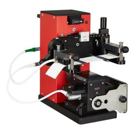
Prediction of the converting properties of paper/board/OPP foils concerning the dimension stability at thermal load up to 230°C.
