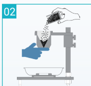
Block the bottom hole of funnel with a dry, clean finger and then add sample
