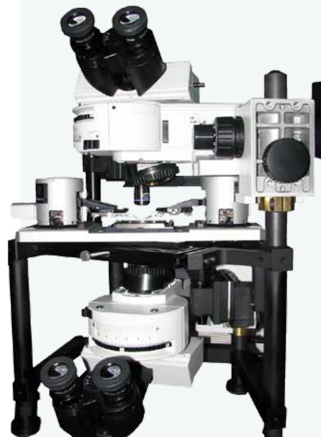
AFM with online water immersion objective for the highest optical resolution and purity
