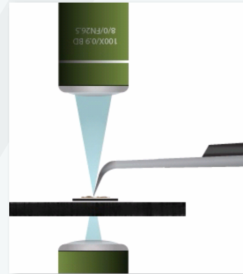
Extended transparent glass probe with high Q Factor
