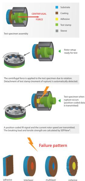
The LUMiFrac is an innovative adhesion analyser, which employs centrifugal forces to determine temperature-controlled tensile as well as shear strength as an absolute physical quantity in N/mm<sup>2</sup>.
