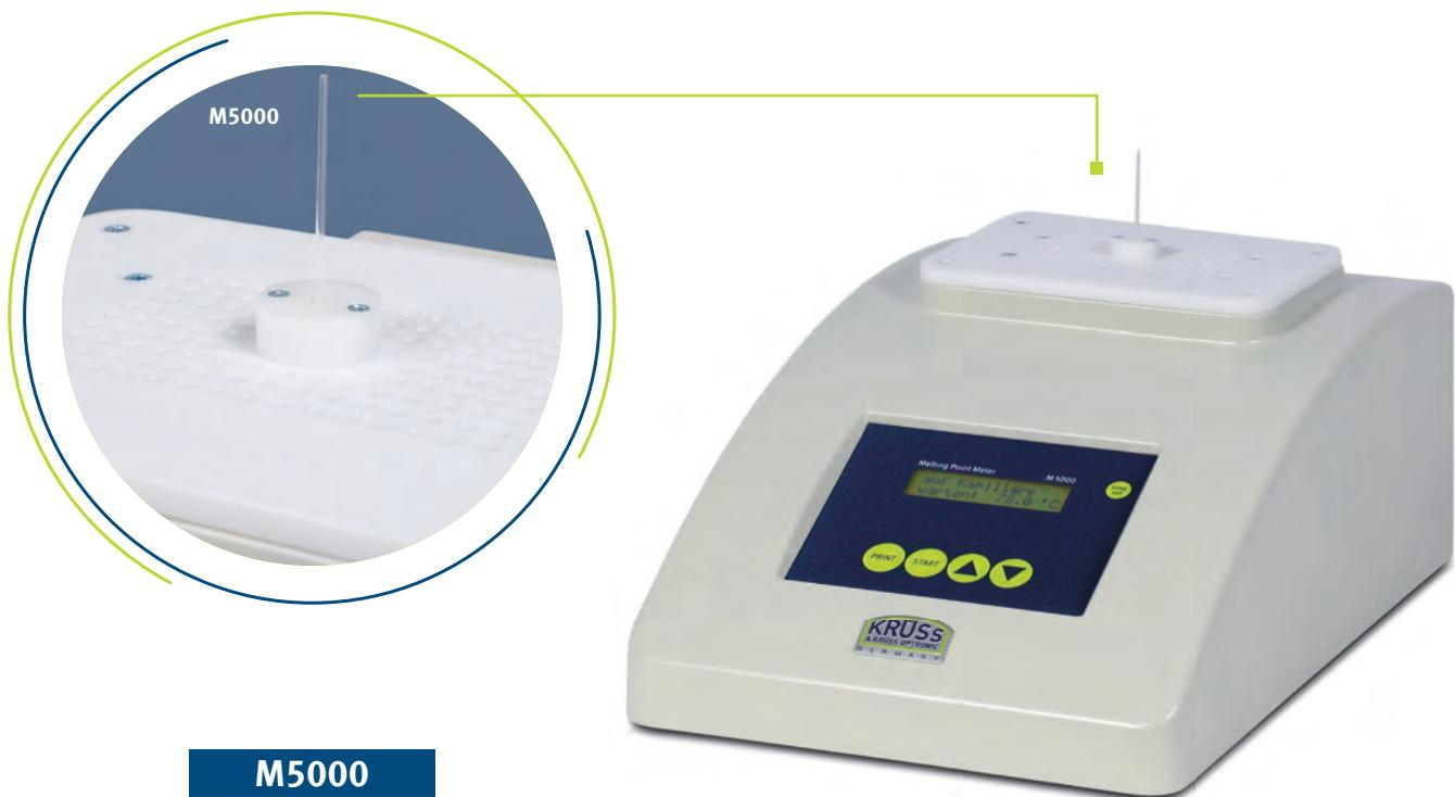
The M5000 provides fast, easy and automatic examination of powdery substances with a melting point up to 400 °C. Due to the automatic determination of the melting point, an objective measurement result is always guaranteed. The high preheating rate and the integrated fan cooling allow fast and reliable measurements in any temperature range. The display provides a well-arranged readout of all important measuring data.
