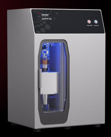
The Guarded Heat Flow Meter (GHFM-01) adheres to ASTM E1530 standards for accurately measuring thermal resistance and thermal conductivity of solids like metals, polymers, composites, and pastes.
