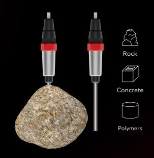
Transient Line Source (TLS-150 mm) Sensor
