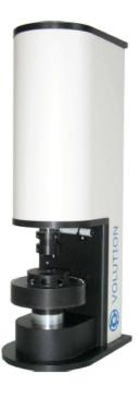
**Flowability of Powder under Load:** measurement in ring shear cells is used to determine flowability data according to the Mohr-Coulomb model. The resulting values can be used for designing silos or to predict powder flow under load.
