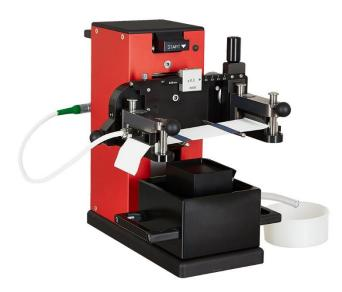
Measurement of the dynamics of the change in dimension of paper by means of one-sided contact with water or water based liquids under adjustable tension
